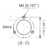
Each level is supplied outfitted with screws and oiltight gasket
