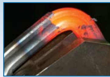
Nickel Chrome plated industrial rails are heat formed from cold drawn profiled steel
