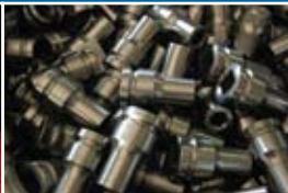
S.A.E. 4140 Chrome Molybdenum steel sockets - Ready for black phosphate finishing
