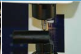
Each production run is tested for correct HRC hardness
