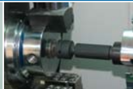
Each production run is torque tested on automatic test beds
