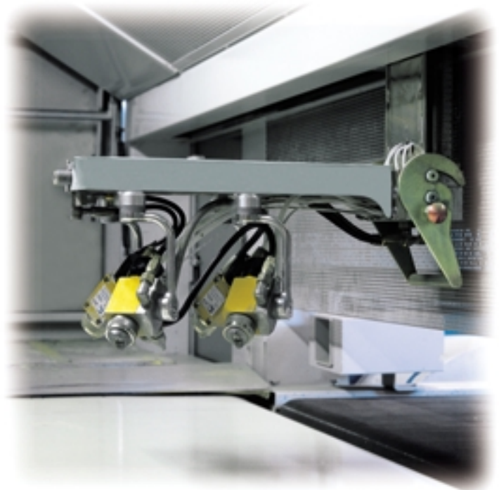
Multiconnection for robotized painting lines.
