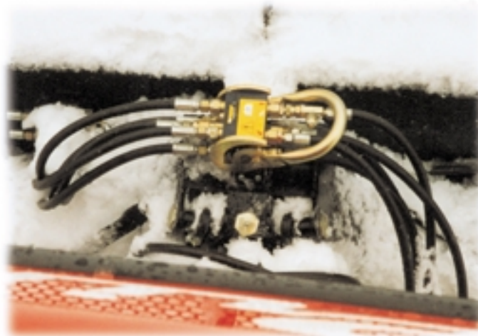
Quick connection for hydraulic snow-ploughs.
