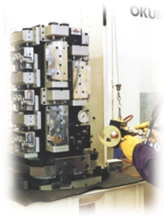
Multiconnection for machining centers. Loaded pallet ready for connection.
