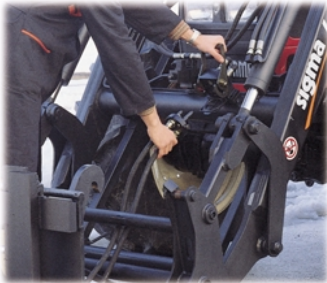
Hydraulic connection for front loader attachments.
