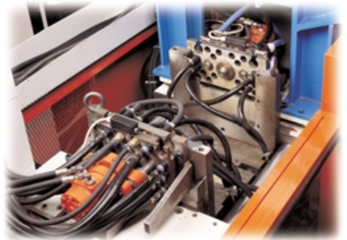
Multiconnection for quick moulds replacement. Moulding machine. Up to 18 hydraulic, electrical and pneumatic lines.
