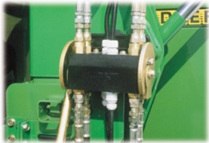
Simultaneous multiple connection up to 12 hydraulic, electrical and pneumatic lines without oil spillage.
